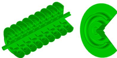
Figure 5: Choke mode structure.
