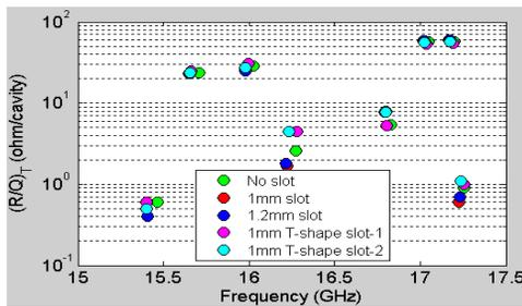
Figure 4:  $(R_T/Q)_T$  for dipole modes.
