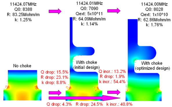
Figure 6: Results for single cell choke mode structure.
