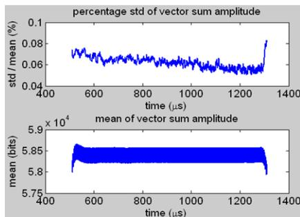
Figure 1: PSD and mean VS amplitude for the flattop.
