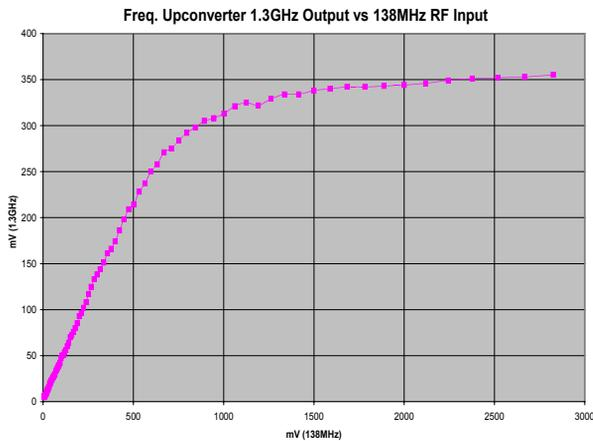
Figure 4: 1.3 GHz Up-converter Response.
