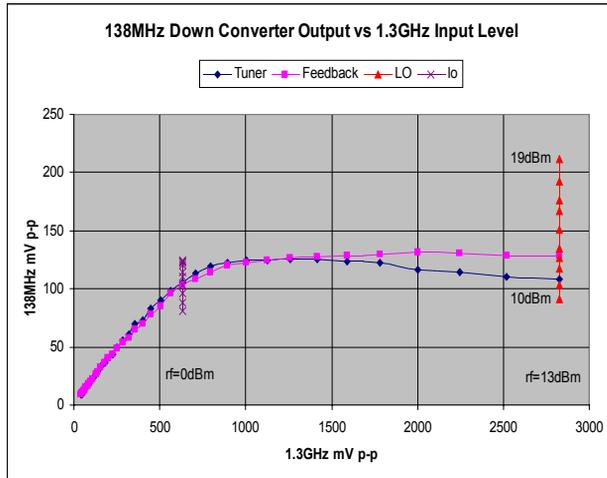
Figure 3: 138 MHz Down-converter Response.
