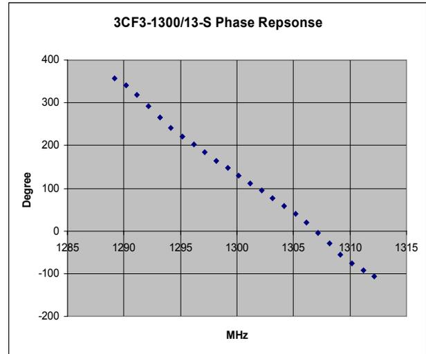
Figure5: 1.3GHz Bandpass Filter Phase Response.
