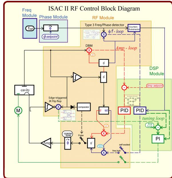
Figure 1: Superconducting Control.
