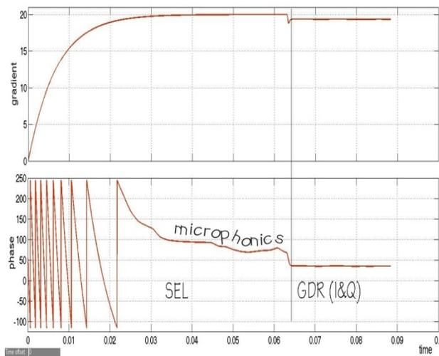
Figure 3: Cavity turn-on process
