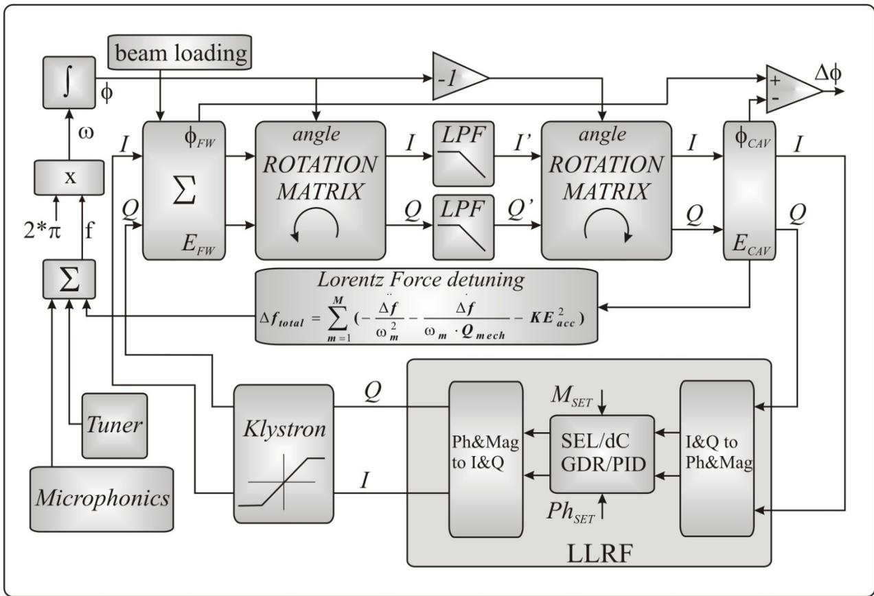
Figure 1: Diagram of the RF System model
