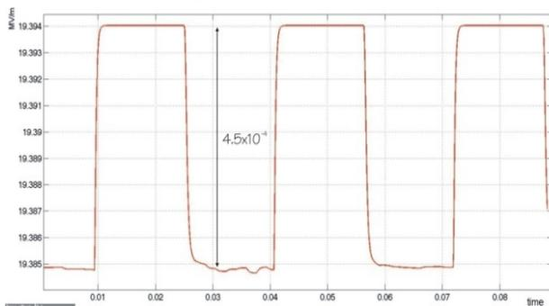
Figure 4: Stabilized cavity gradient for 23 Hz square wave detuning and loop gain of 32.
