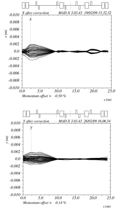
Figure 5: The particle trajectory after correction when random errors are assumed for magnets in BTS transfer line. Top: horizontal orbit, bottom: vertical orbit.
