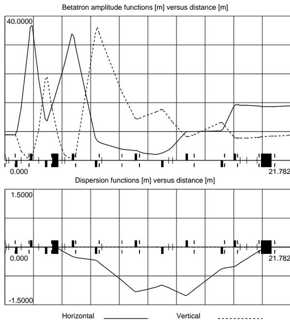
Figure 2: Optical functions of LTB transfer line.
