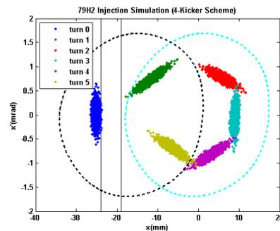
Figure 6: The horizontal phase space at the injection point of storage ring. The injected beam is depicted by blue color, and the beam distribution in subsequent turns in the storage ring are labeled by other color as shown in the legend.
