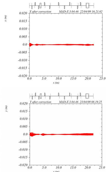
Figure 3: The simulated particle trajectories with random errors after correction in LTB transfer line. Top: horizontal orbit, bottom: vertical orbit.
