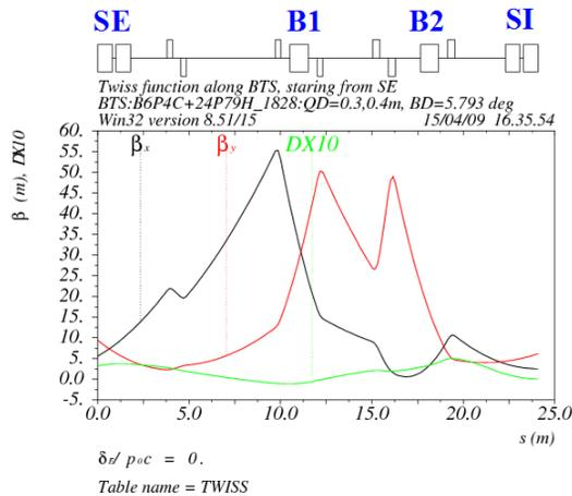
Figure 4: The lattice of BTS transfer line. The dispersion function has been magnified by 10 times for view purpose.
