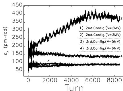
Figure 3(b): The equilibrium vertical emittances for the 2<sup>nd</sup> and 3<sup>rd</sup> configurations for various deflecting voltages. The interior sextupoles were switched on.
