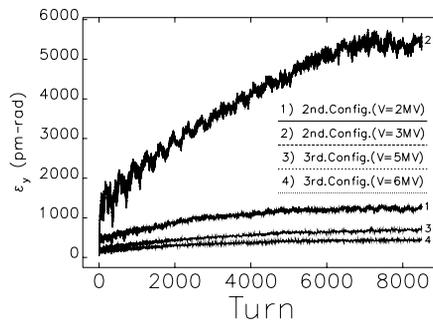
Figure 3(a): The equilibrium vertical emittances for the 2<sup>nd</sup> and 3<sup>rd</sup> configurations for various deflecting voltages. The interior sextupoles were switched off.
