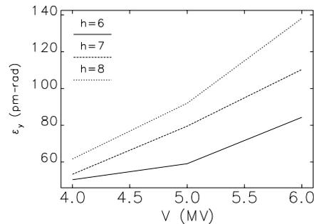
Figure 4(b): The eventual vertical emittances in the 3<sup>rd</sup> configuration versus the deflecting voltages for various harmonics. The interior sextupoles were switched on.
