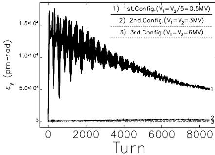
Figure 2: The equilibrium vertical emittance for all three configurations. The deflecting voltages of the first and second cavities are equal for both 2<sup>nd</sup> and 3<sup>rd</sup> configurations but for the 1<sup>st</sup> configuration, the first cavity voltage is one fifth of the second. The interior sextupoles were switched on in between the cavities.
