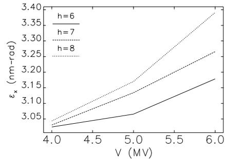
Figure 4(a): The eventual horizontal emittances in the 3<sup>rd</sup> configuration versus the deflecting voltages for various harmonics. The interior sextupoles were switched on.
