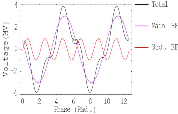
Figure 2: The electron bunch position in the wave form with double RF system. The phase and voltage of harmonic system are adjusted to lengthen the electron bunch.
