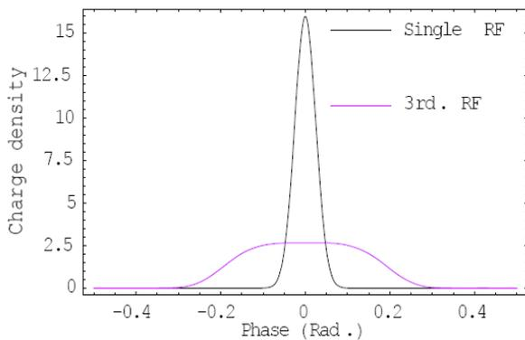
Figure 4: Longitudinal distribution for single and third harmonic system with 3MV gap voltage.
