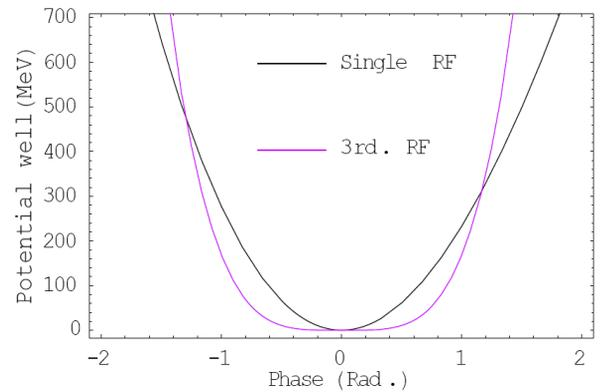
Figure 3: Potential well for single and third harmonic RF system.
