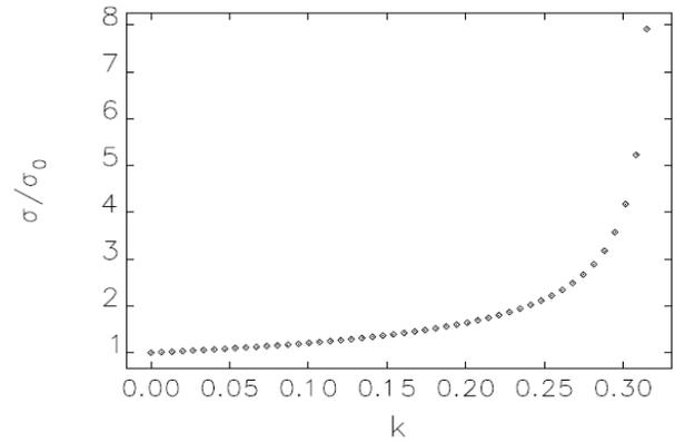
Figure 5: Normalized bunch length versus  $k$  ( $k = V_{HRF}/V_{RF}$ ) for third harmonic RF systems. The main gap voltage is 3 MV.
