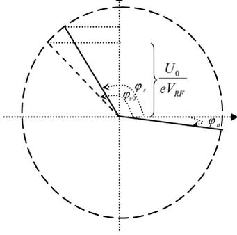
Figure 1: The synchronous phases for single and double RF systems,  $\varphi_s < \varphi_{s0}$ .
