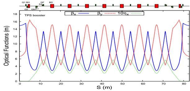
Figure 7: Lattice optical functions of the TPS booster ring.
