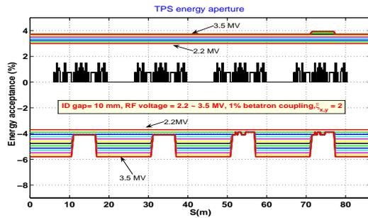
Figure 3: Energy aperture for RF gap voltage from 2.2 MV to 3.5 MV (larger aperture) with vertical chamber full gap of 10 mm in the ID straights and 1% betatron coupling. 6-D particle tracking is performed with TRACY-II. Chromaticities are set to 2.0 in both planes.
