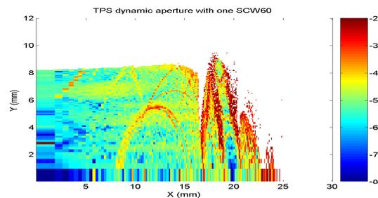
Figure 5: Dynamic aperture at long straight center with one SCW60 putting in one short straight (1-m off straight center). Chamber full size of the wiggler is 40 x 11 mm<sup>2</sup>.
