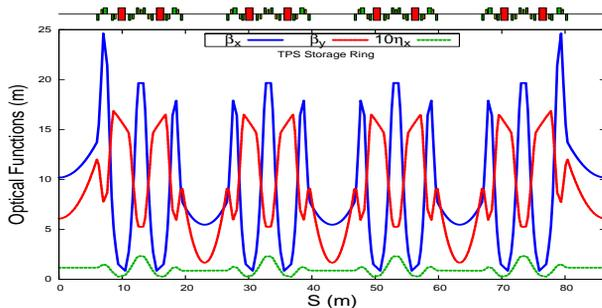
Figure 1: Lattice optical functions of the TPS storage ring.
