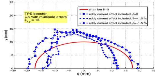
Figure 8: Dynamic aperture at the long straight center of the TPS booster with magnetic multipole errors. The bore radius of the quadrupoles and sextupoles is 18 mm.
