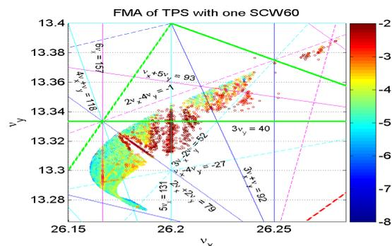
Figure 6: Corresponding frequency map with one SCW60. One of dangerous resonance lines is  $2v_x + 2v_y = 79$  that causes a big dip.
