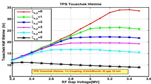
Figure 4: Estimated Touschek beam lifetime as a function of RF gap voltage for different chromaticity settings using TRACY-II and Piwinski formula. Bunch current 0.5 mA, ID vertical chamber size 10 mm and betatron coupling 1% assumed in the simulations.
