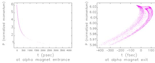
Figure 4: The temporal phase space at the entrance and the exit of alpha magnet.
