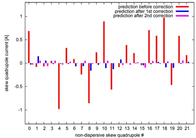
Figure 3: Skew quadrupoles currents for three iterations of the betatron coupling correction procedure involving three subsequent orbit response matrix measurements. The maximum applied skew quadrupole strength  $|k_s|$  of  $\approx 0.004$   $\text{m}^{-1}$  corresponding to  $\approx 1$  A stays well below the maximum of  $0.03$   $\text{m}^{-1}$  at 7 A.
