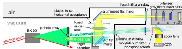
Figure 5: Layout of the high resolution emittance measurement beam-line operated at the central dipole ARIMA-BX-09, showing the X-ray branch with pinhole array and the vis-UV branch [8][9].
