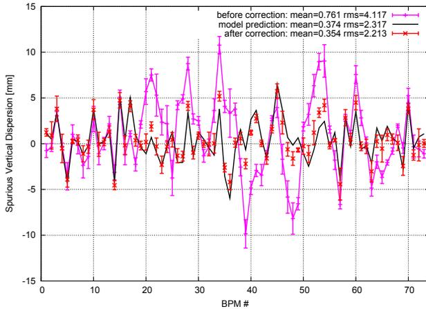
Figure 2: The setting for six dispersive ( $\eta_x \approx 0.3$  m) skew quadrupoles is determined by an SVD fit to the measured spurious vertical dispersion  $\eta_y$  (magenta points +) without any weighting factor cut. It reduces the initially measured  $\eta_y$  of 4.1 mm to 2.2 mm RMS (red points  $\times$ ). The model prediction (black line) is given for comparison indicating that a significant further reduction of  $\eta_y$  is not possible utilizing those six knobs.
