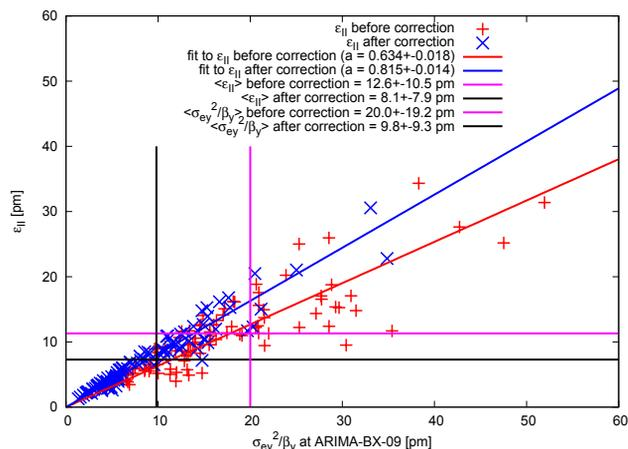
Figure 6: Simulation result for 100 randomly distorted SLS lattices. Shown is  $\epsilon_{II}$  vs.  $\sigma_{ey}^2/\beta_y$  before (red points +) and after coupling correction (blue points x) utilizing 22 non-dispersive skew quadrupoles. Both quantities  $\sigma_{ey}^2/\beta_y$  and  $\epsilon_{II}$  are clearly reduced (magenta compared to black lines) and appear to be highly correlated after the applied coupling correction.
