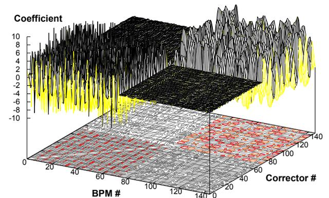
Figure 4: Coupled BPM/Corrector response matrix after the application of two successive betatron coupling correction steps. The RMS of the coupling terms has been reduced by a factor  $\approx 2.2$ .
