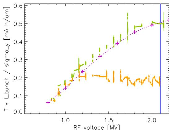
Figure 1: Measurement of beam lifetime (normalized to beam height and bunch current) as a function of RF voltage: the upper (green) and lower (orange) data points were respectively measured with optimum and zero settings of the skew quadrupoles and auxiliary sextupoles. The crosses connected by the dotted line (purple) are a TRACY 6-d tracking simulation for the ideal lattice. The line at right (blue) marks the RF-voltage as used in normal operation.
