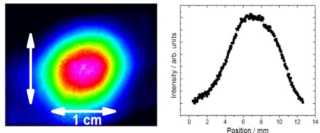
Figure 3: Left: Focus of the THz beamline after mirror M7 (see Fig. 1). Right: Beam profile of the focussed THz radiation.
