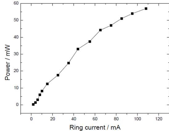
Figure 5: Averaged THz power measured in the focus of the THz beamline. Data were taken in low- $\alpha$  operation at an electron energy of 630 MeV.
