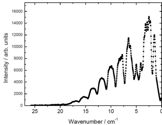
Figure 4: Typical FTIR spectrum at the MLS THz beamline in the low- $\alpha$  mode for 630 MeV. The spectrum is taken in the bursting mode.
