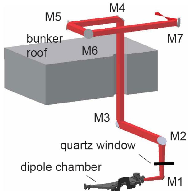
Figure 1: Layout of the MLS THz beamline. For details see text.
