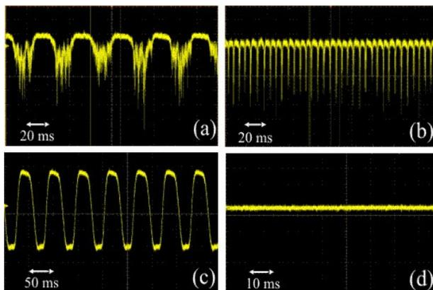
Figure 2: Oscilloscope traces of bursting and stable THz signals at MLS for 630 MeV electron energy, low- $\alpha$  optics, and a cavity voltage of 200 kV measured with an InSb-detector: Bursting at 50 mA ring current: The chopped THz signal amplitude (a) and the unchopped THz signal amplitude (b) show bursting instabilities. Stable THz radiation at 19 mA ring current: The chopped THz signal amplitude (c) and the unchopped THz signal amplitude (d) are constant and show no bursting instabilities.
