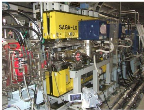
Figure 4: Photograph of the APPLE-II type undulator.
