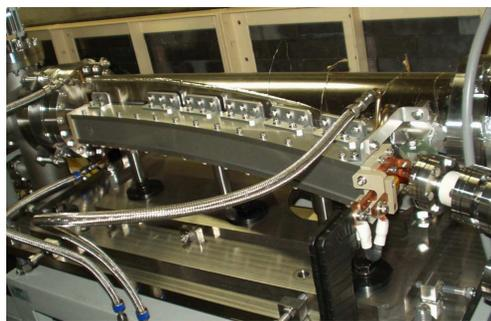
Figure 2: Photograph of the new out-of-vacuum type septum magnet.
