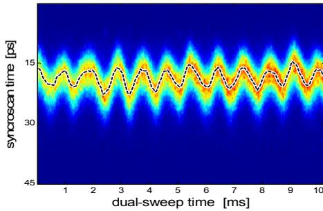
Figure 1: Synchrotron oscillations observed in Hamamatsu C5680 R1 dual scan mode. Fast vertical sweep range is 45ps, slow horizontal sweep time is 10ms.
