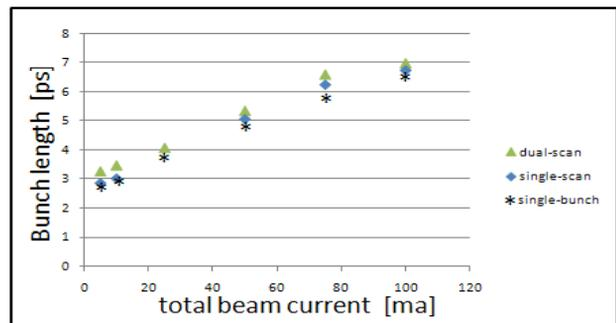
Figure 3: Multibunch fill with single-bunch superimposed.
