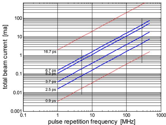
Figure 5: Total beam current vs. pulse rate for the range of bunch lengths corresponding to Fig. 1.
