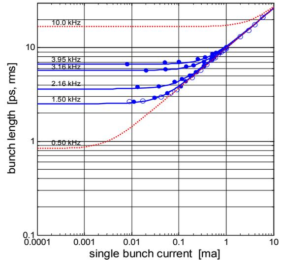
Figure 2: Low- $\alpha$  mode bunch lengthening. 0.5kHz and 10kHz curves extrapolated from Equation 2.
