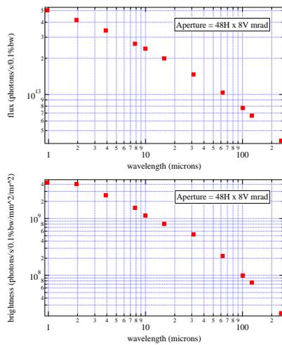
Figure 1: IR flux and brightness for the existing SPEAR3 ID port with a  $8V \times 48H$  mrad<sup>2</sup> aperture for a 100mA beam.
