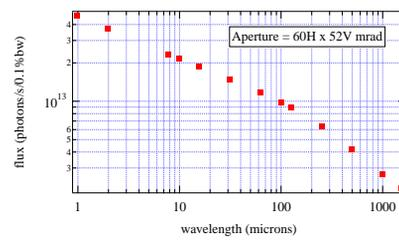
Figure 2: IR flux for a potential SPEAR3 dipole port with a  $60H \times 52V$  mrad<sup>2</sup> aperture for a 100mA beam.
