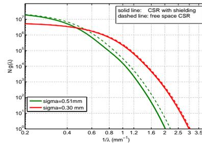
Figure 5: The CSR amplification factor  $Ng(\lambda)$  for SPEAR3 in two different  $\alpha$ -values for corresponding single bunch currents just below the bursting threshold. The rms bunch length for SPEAR3 achromatic lattice is 5.1 mm.
