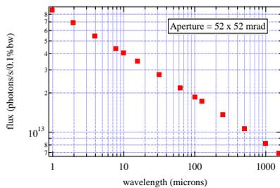
Figure 4: Flux collected by the  $52 \times 52$  mrad<sup>2</sup> from the chicane magnet for a 100 mA beam.
