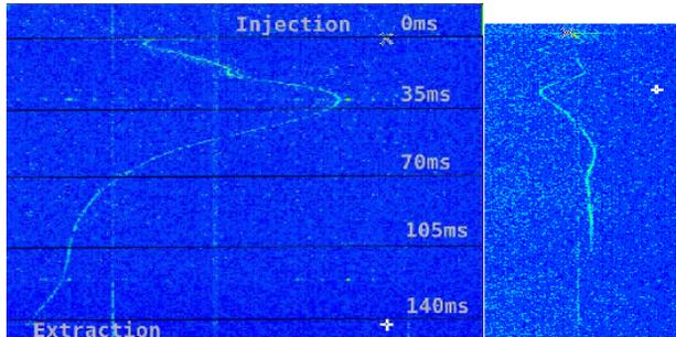
Figure 1: Uncompensated (left) and quite compensated (right) tune shifts during booster cycle. Tunes are shown as continuous curves.
