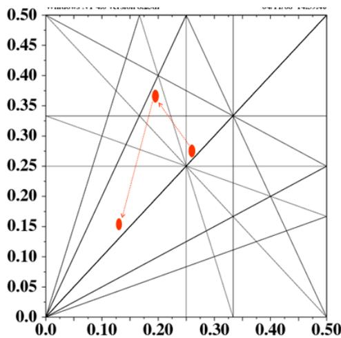
Figure 2: Booster tune diagram and tune shifts during a fully uncompensated cycle.
