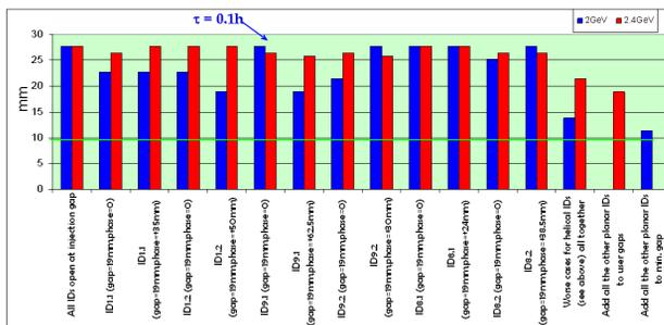
Figure 5: Aperture studies with and without insertion devices at both 2 GeV (blue bars) and 2.4 GeV (red bars)
