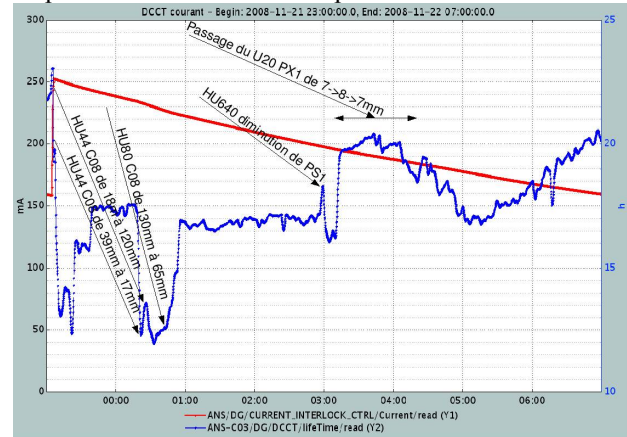
Figure 2: Beam lifetime fluctuations due to ID gap changes.
