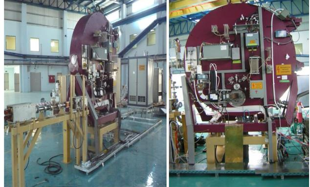
Figure 1: The BESSY I Microtron installed in the SESAME experimental hall.
