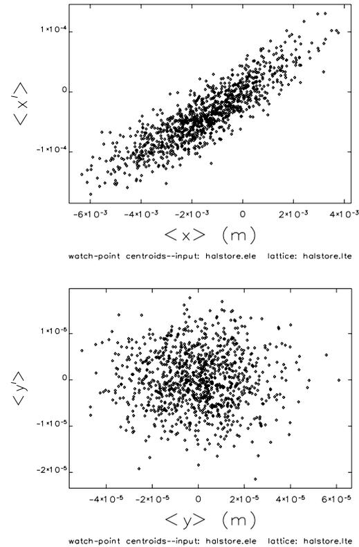
Figure 4: Particle tracking of storage beam under different injection system errors for the 1000 random seeds.
