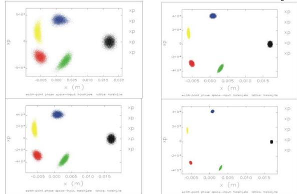
Figure 3: Particle tracking for the different emittance injected beams. Left up: 50nm-rad, left down: 20nm-rad, right up: 5nm-rad, right down: 1nm-rad.
