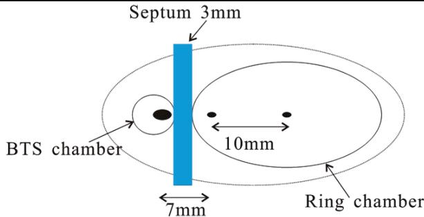
Figure 2: Setup of bump and septum.
