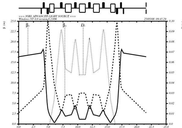
Figure 1:  $\beta$  and dispersion functions of one cell.
