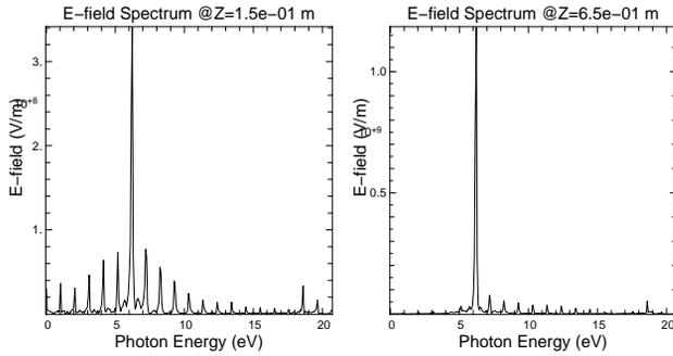
Figure 1: On-axis electric-field spectrum  $|E(\omega)|$  at  $z = 0.15$  m (left plot) and  $z = 0.65$  m (right plot) from an electron beam sub-harmonically bunched at  $\lambda = 1200$  nm in an undulator resonantly tuned to  $\lambda_R = 200$  nm ( $\hbar\omega = 6.1$  eV). In addition to strong sideband emission early in  $z$  whose blueward components persist later in  $z$ , there is also evident third harmonic emission at 18 eV.
