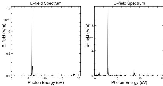
Figure 3: On-axis electric-field spectrum  $|E(\omega)|$  from (left) a "normal", single frequency undulator with  $a_{u,1} = 1.0$  and (right) a biharmonic undulator with  $\lambda_{u,2} = 3\lambda_{u,1}$ ,  $a_{u,1} = 1.0$  and  $a_{u,2} = 1.5$ .
