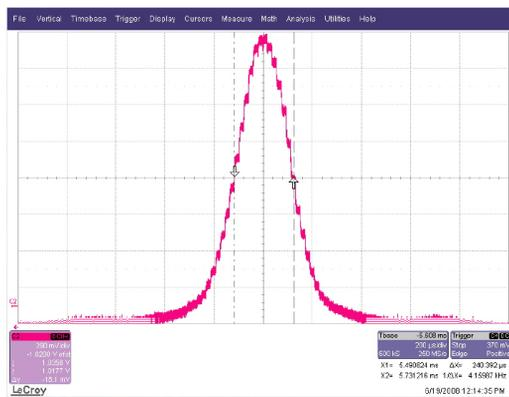
Figure 3: Measurement results of autocorrelator. FWHM= 0.240ms, De-convoluted pulse width FWHM ~ 85fs.
