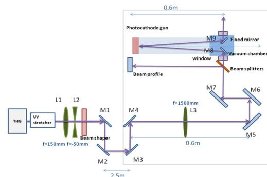
Figure 6: Schematic of beam transport.
