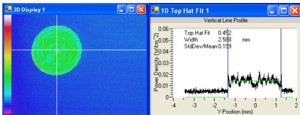
Figure 8b: Laser beam profile after spatial shaper.
