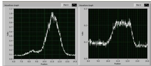
Figure 9: Laser pulse profile before and after pulse stacking.
