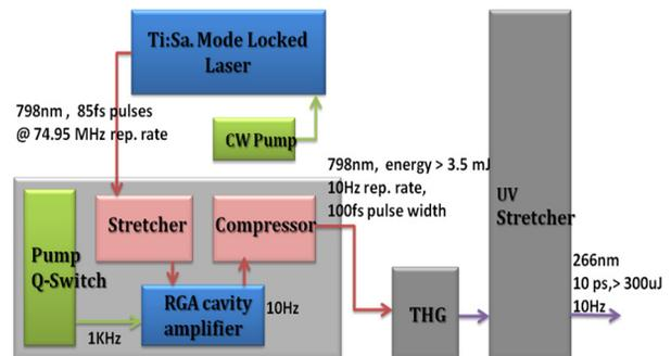
Figure 1: Layout of ultrafast laser system.
