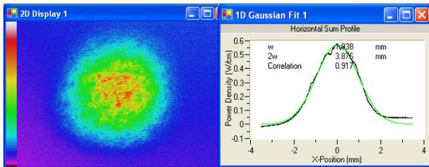
Figure 8a: Laser beam profile before spatial shaper.
