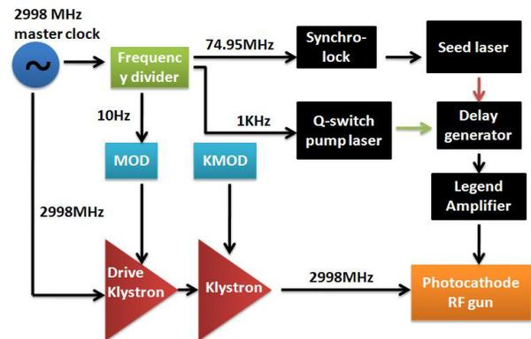
Figure 5: Schematic of synchronization system.
