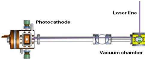
Figure7: Schematic of laser beam couple to cathode.
