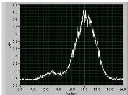
Figure 4: Measurement results of UV crosscorrelator. FWHM = 1.7mm, UV pulse width = 11ps.
