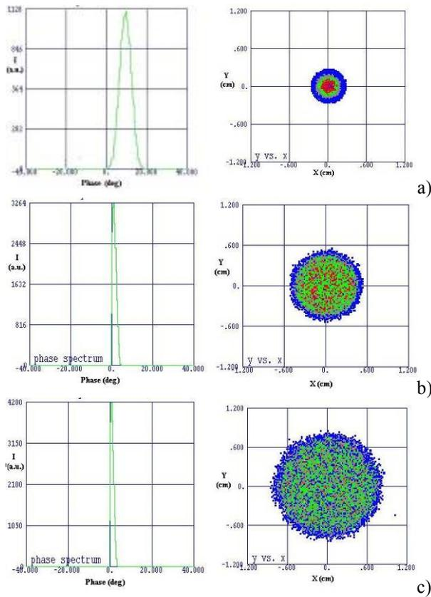
Figure 3: PAMELA simulation results of electron bunch a) at entrance of Acc. cavity, b) at exit of Acc. cavity, c) at entrance of undulator. Left and right frames, respectively: longitudinal profile and transverse profile.
