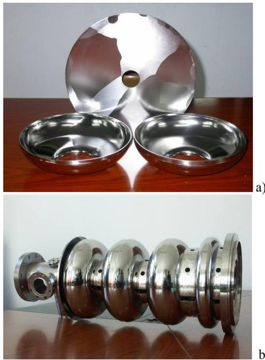
Figure 2: a) large grain niobium sheet and half-cell cavity
