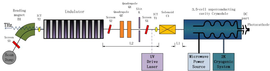
Figure 1: Schematic layout of the PKU Terahertz Facility.
