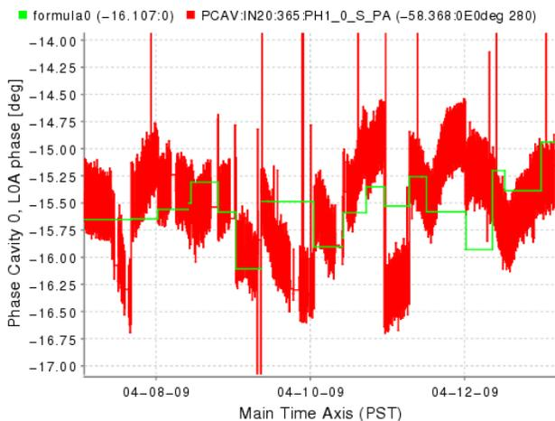
Figure 3: Beam phase (red) and L0A klystron phase (green) vs time. Beam phase is monitored continuously, while the klystron phase changes only after phasing.
