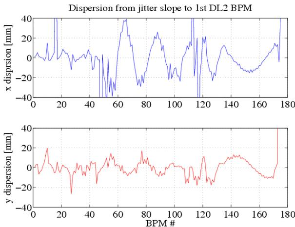
Figure 7: Dispersion derived from jitter measurement. Some  $x$ -dispersion is not contained in BC2 but leaks out and is about 10 mm in the undulator region.
