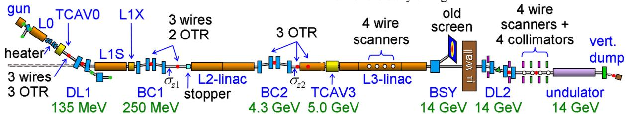
Figure 1: LCLS schematic layout of the Linac sections (L0, L1, L2, and L3) with the two bunch compressors (BC) followed by a dog leg (DL2) and some collimation before reaching the undulator and dump.
