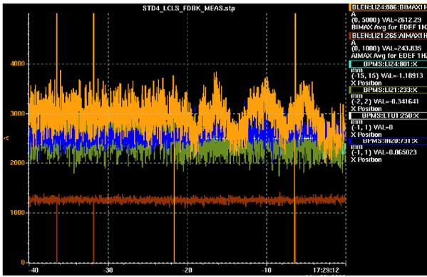
Figure 6: Medium term (5 min) oscillation of 25% of the BC2 peak current around 3000 A when the bunch length feedback is switched off.
