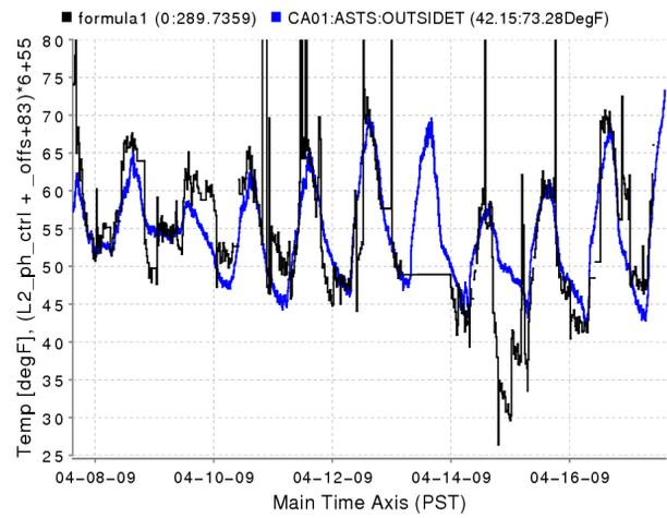
Figure 2: Outside temperature changes (blue) and overlaid the L2 phase (black, multiplied by 6).
