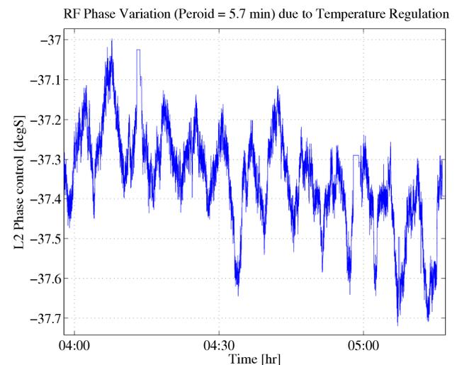
Figure 5: Medium term (5 min) variation of the L2 phase of  $0.4^\circ$ . The phase is controlled by a beam based feedback stabilizing the bunch length signal after BC2.
