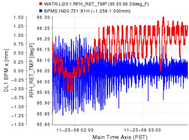
Figure 4: Small, but oscillating temperature variations of  $\pm 0.1^\circ\text{F}$  caused energy jitter due to not tightened RF cables.
