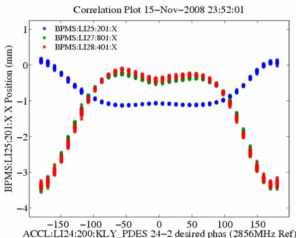
Figure 1: RF kick for  $360^\circ$  phase change of klystron 24-2.
