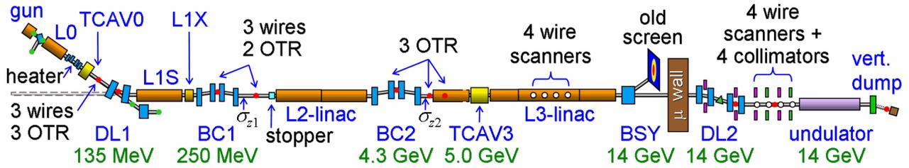
Figure 3: LCLS schematic layout of the Linac sections (L0, L1, L2, and L3) with the two bunch compressors (BC), followed by a dog leg (DL2) and some collimation before reaching the undulator and dump.
