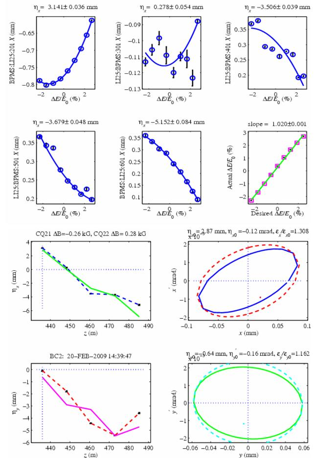
Figure 5: Results of a dispersion measurement at BC2.
