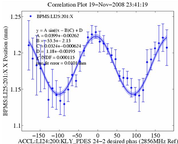
Figure 6: RF kick for 360° phase change of klystron 24-2 after an orbit bumps around the structure reduced the kick.
