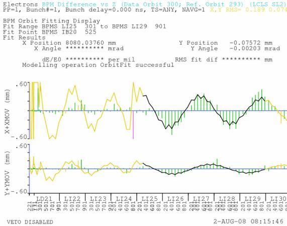
Figure 4: Difference orbit is plotted with the klystron 25-7 off (minus on). An oscillation starts right there indicating an RF kick. The signed “amplitude” is  $-0.4$  mm in  $x$ .
