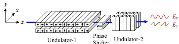
Figure 1: A sketch of crossed undulators for polarization control.
