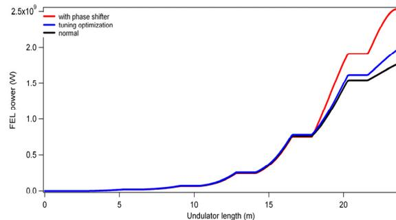
Figure 5: FEL power along the undulator for a standard radiator (black) and for a radiator with a proper set of the phase shifters (blue and red lines), in order to compensate the detuning.
