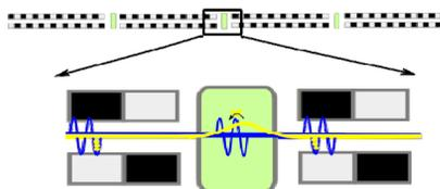
Figure 1: Sketch of a typical undulator chain for high gain FELs. Phase shifters (green box) allow controlling the slippage between electrons and the FEL radiation in the breaks.
