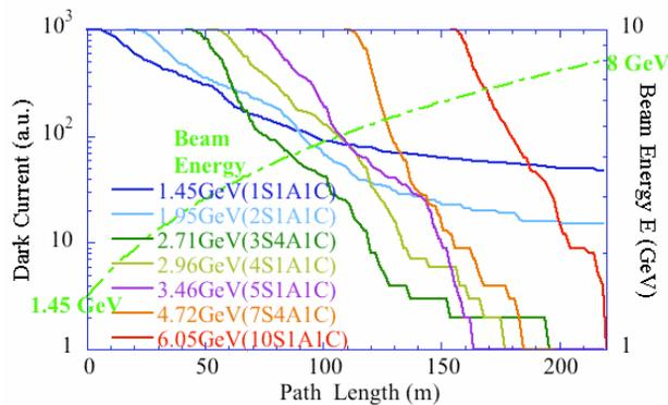
Figure 5: Dependence of the dark current decay on the emission-position along the linac with additional sextupoles. The seven different coloured lines represent the same conditions as in Fig. 3.
