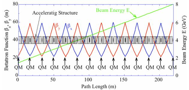
Figure 2: Beam envelope over the C-band main linac. The symbol QM represents a quadrupole magnet.
