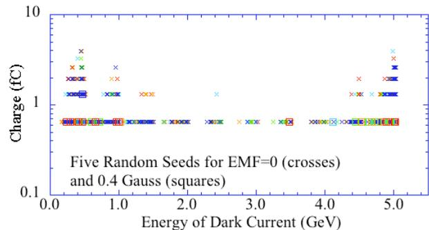
Figure 7: Energy spectra of dark currents in the undulator hall with and w/o EMF.
