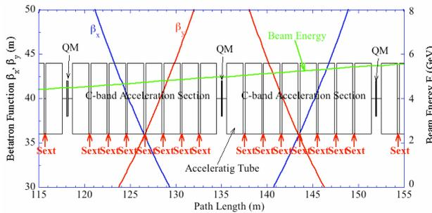
Figure 4: Sextupole magnet arrangement for enhancement of the dark current decay.
