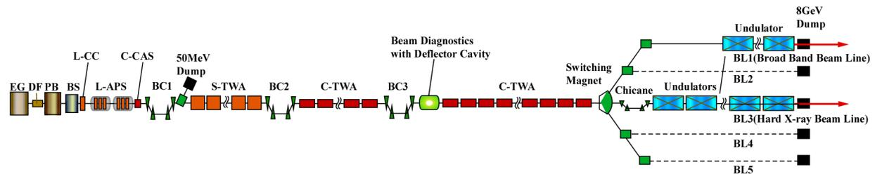
Figure 1: Schematic drawing of the XFEL accelerator system. EG, 500-kV electron gun; DF, deflector with collimator; PB, 238-MHz pre-buncher; BS, 476-MHz booster; L-CC, L-band correction cavity; L-APS, L-band alternating periodic structure; C-CAS, C-band correction accelerating structure; BC1~3, bunch compressor1~3; S(C)-TWA, S(C)-band travelling-wave structure; BL, beam line.
