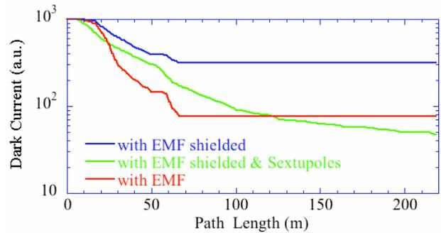
Figure 6: Dark current decay along the linac under three different conditions. The dark emission-point is the 1<sup>st</sup> cell of the 1<sup>st</sup> accelerating structure in the 1<sup>st</sup> C-band section.
