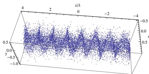
Figure 2: Section of e-beam calculated in TREDI for the parameters in Table 1 at the undulator exit.
