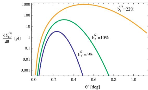
Figure 5: Calculated angular CTR distribution for the bunching factors predicted by simulations in Fig 4, for different harmonics (upper index) of the  $10.6 \mu\text{m}$  microbunching wavelength and different helical modes (lower index).
