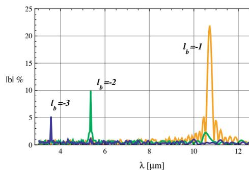
Figure 4: TREDI: Spectrum of the microbunching wavelength  $\sim 10$  cm from the undulator exit with 50000 particles.
