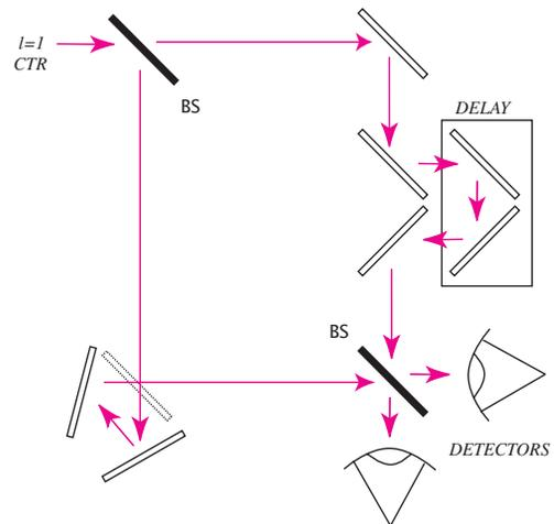
Figure 7: Simple interferometric scheme for resolving helical optical phase in the CTR. The mirror in the bottom left (dashed) is removable, allowing one path to experience either a single or a double reflection before encountering the second beam splitter (BS).
