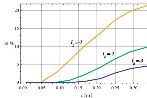
Figure 3: TREDI: Evolution of the azimuthal mode bunching factors along the interaction length. The undulator exit is at  $\sim 26$  cm, after which the drift allows the velocity modulation to turn into density modulations, and the bunching factors continue to increase.
