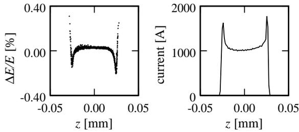
Figure 2: Longitudinal phase space and current distribution after bunch compression, acceleration to 1.7 GeV, and passage through a 3-stage beam spreader with a low value of  $R_{56}$ . The tail is on the right.
