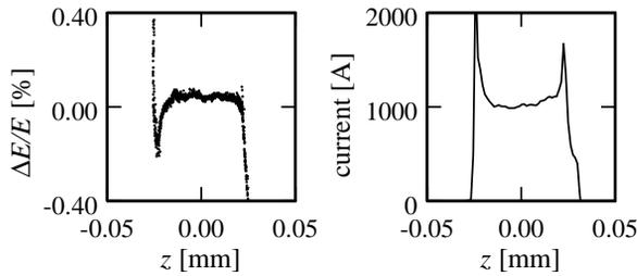
Figure 5: Longitudinal phase space and current distribution after bunch compression, acceleration to 1.7 GeV, and passage through the low- $R_{56}$  beam spreader, with overestimated shot noise.
