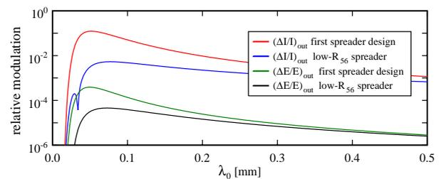
Figure 4: Relative current and energy modulations at the exit of the spreader tree from amplified shot noise, versus initial wavelength  $\lambda_0$ . Analytic calculations for linear amplification are shown for the first spreader design and the low- $R_{56}$  design.
