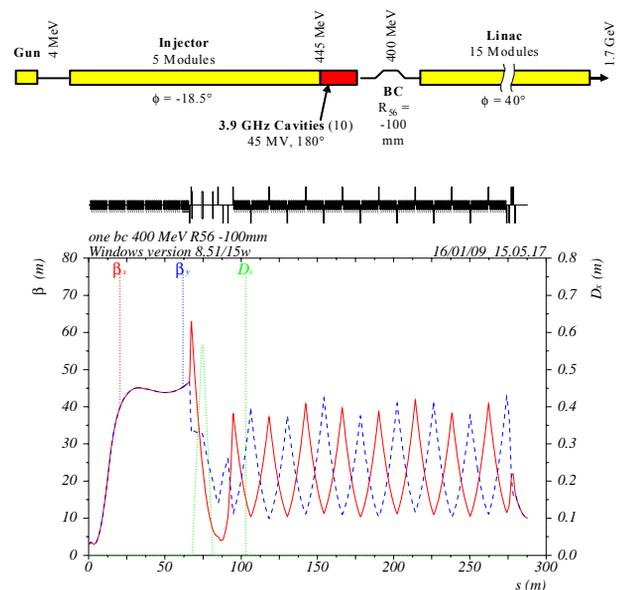
Figure 1: Schematic diagram and lattice functions of the single-stage bunch compressor.
