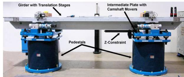
Figure 1: Complete SMS, showing all major components.
