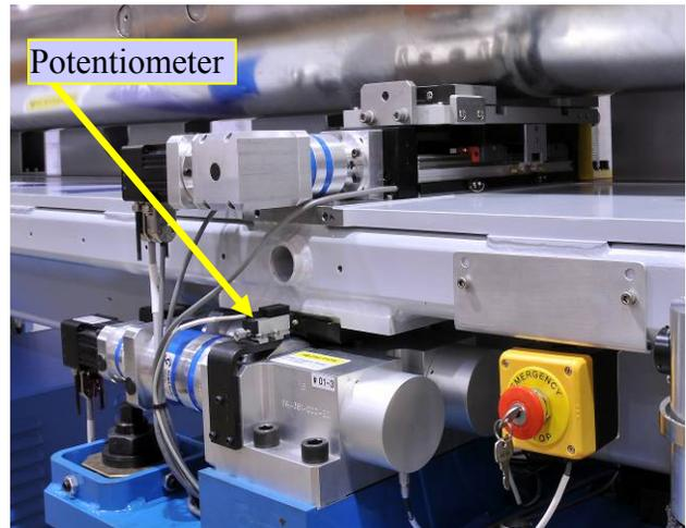
Figure 4: The girder, an E-stop button, a double camshaft mover with motors and potentiometer on an intermediate plate, and a translation stage with motor are shown.
