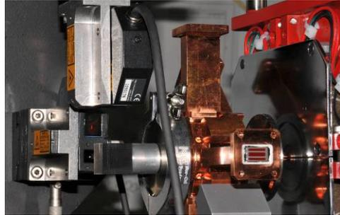
Figure 3: Two Keyence sensors and precision cube.
