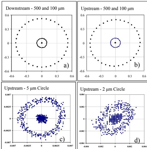
Figure 5: Girder displacement tests show excellent SMS reproducibility, repeatability, and stability.
