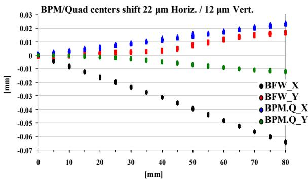
Figure 6: BPM and quadrupole magnet centers shift 22 microns horizontally and 12 microns vertically when the undulator is moved out of the beamline by 80 mm, but return to zero within two microns when it moves back in.
