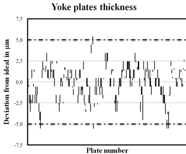
Figure 4: Manufacturing accuracy of 204 yoke plates, on the vertical axis is shown the deviation with respect to the ideal thickness of 7.5 mm.
