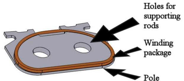
Figure 3: 3D model of one of the 408 plates constituting the two magnet yokes. Each plate includes a pole and a superconducting coil winding.
