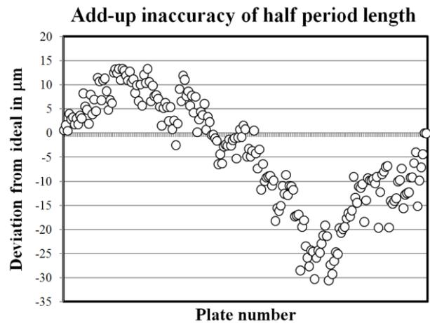
Figure 5: Add-up inaccuracy of the period length after yoke stapling and pressing.
