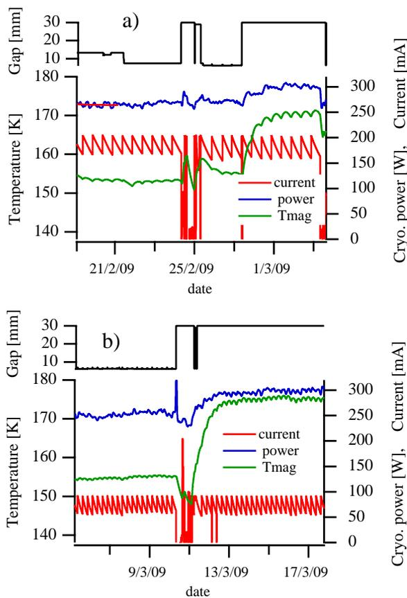
Figure 2: Average temperature of the CPMU (Green) and power extracted from the cryogenic loop (blue) versus time in 7/8 filling pattern, 200mA (a) and 16 bunch mode, 90mA (b). The beam current is shown in red and the undulator gap in black.
