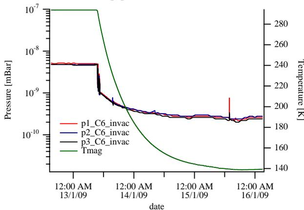
Figure 4: Evolution of the residual pressure seen from the three penning gauges installed on the CPMU during a cooling phase. The average temperature of the undulator (Tmag) is shown in green.
