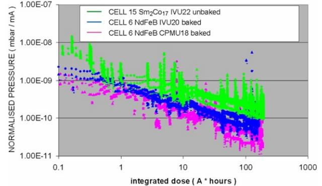
Figure 5: Dynamic pressure in mbar/mA versus integrated current for three different in-vacuum undulators: Cell 6 CPMU (pink), cell 9 IVU20 (blue) and cell 15 IVU22 (green).
