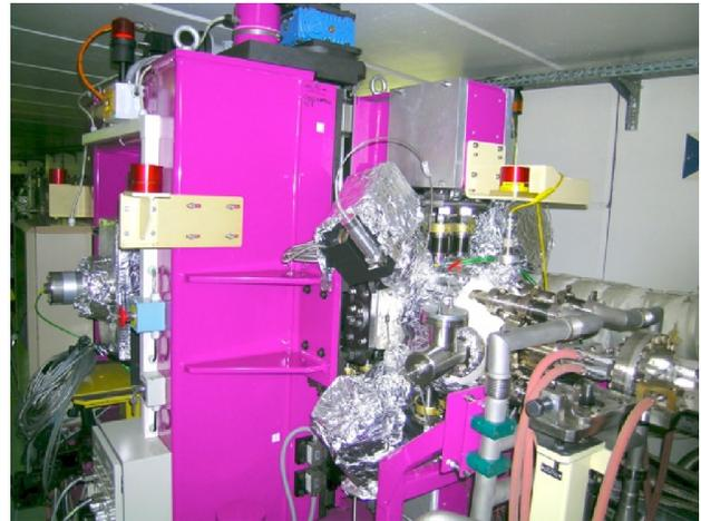
Figure 1: First CPMU prototype installed in the ESRF ID6 straight section.
