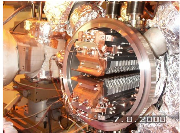
Figure 3: CPMU opened at the entrance for the installation of a flexible thermal connection (August 2008).
