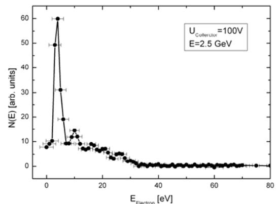
Figure 2: Spectrum of the energy of low energy electrons inside the vacuum system of the ANKA storage ring at a beam energy of 2.5 GeV.
