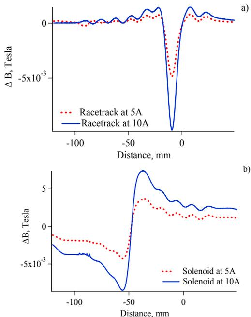
Figure 1: Efficiency of the racetrack (above) and solenoid (below) field at two different currents on the background field of the main coil powered with 50 A current.
