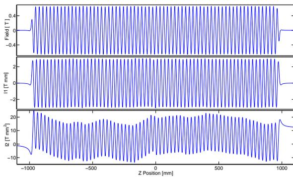
Figure 2: Preliminary Hall-probe measurements for U32 (12 mm gap) and corresponding field integrals.
