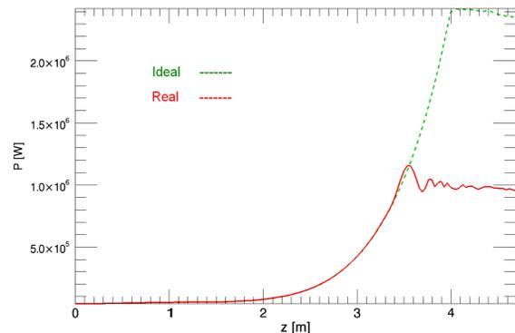
Figure 7: Simulated power gain curve for an HHG seed to the electron beam at the entrance of U33. For presently deteriorated field, the output power is affected by a factor of two with respect to the ideal case.
