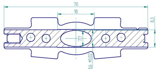
Figure 1: Cross-section of the undulator vacuum chamber.
