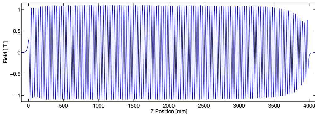
Figure 5: Field decay of up to 40% is observed at the edges of U33. This is a measurement with 9 mm gap size.
