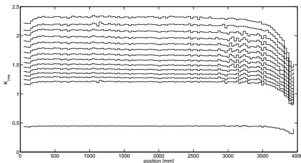
Figure 6: Measured  $B_y$  is used to plot variation of the undulator parameter  $K_{rms}$  along the device for different gaps. The top curve is for 9 mm gap size, the next curves are for larger gaps increasing in 0.5 mm steps up to 15 mm, the last one corresponds to 25 mm.
