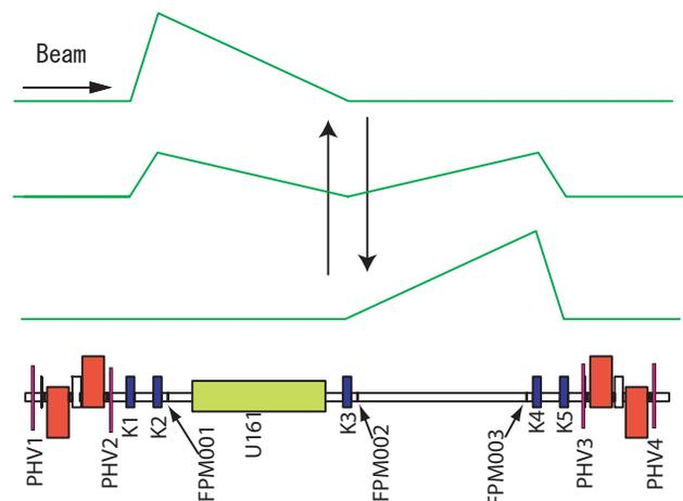
Figure 6: Schematic drawing of the angular bump and magnets and BPMs layout. The bump sinusoidally switched.
