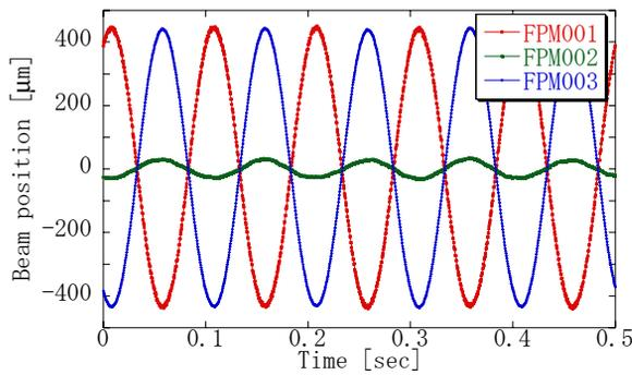
Figure 7: Horizontal beam positions at a switching frequency of 10Hz. Monitors were placed inside the bump section.
