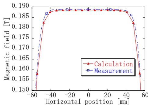
Figure 3: Typical horizontal distribution of the magnetic field. Solid blue line and red crosses show the results of the measurement and the calculation, respectively.
