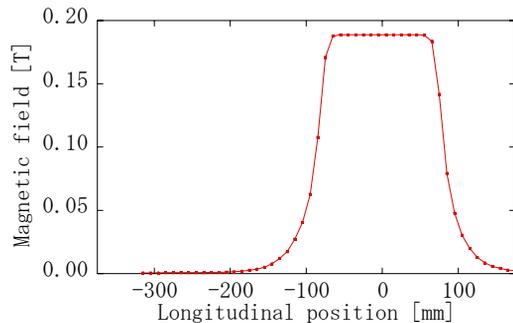
Figure 4: Typical longitudinal field distribution of the magnetic field.
