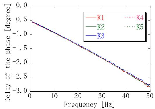
Figure 5: Phase delay as a function of the frequency. These lines represent the phase delay between input signal and magnetic field.
