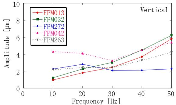
Figure 11: Vertical oscillation amplitude as a function of the switching frequency detected using five Fast BPMs.
