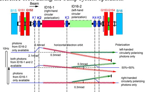
Figure 1 : Schematic drawing of the conceptual design for producing the fast helicity switching variable polarized photon.
