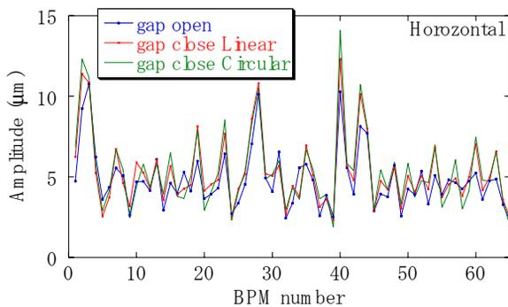
Figure 8: Horizontal oscillation amplitude at a switching frequency of 0.1Hz. Monitor was placed whole ring out of bump section.
