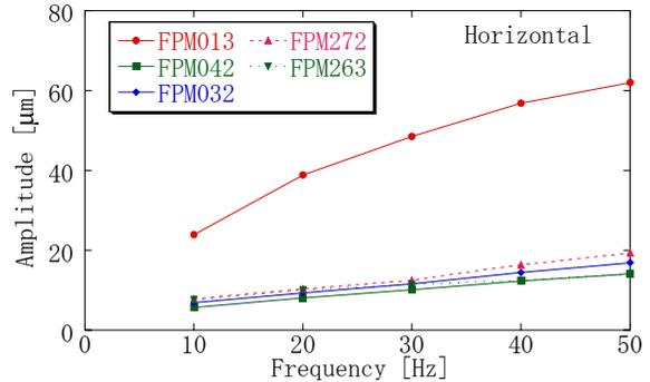
Figure 10: Horizontal oscillation amplitude as a function of the switching frequency detected using five Fast BPMs.
