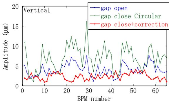
Figure 9: Vertical oscillation amplitude at a switching frequency of 0.1 Hz. Monitor was placed whole ring out of bump section.
