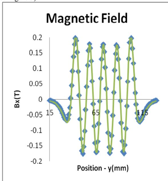
Figure 3: Comparison of magnetic field in simulation and measurement: Radia simulation is graphed in solid line, and magnetic probe measurement in the middle of the undulator is graphed in blue rhombuses.
