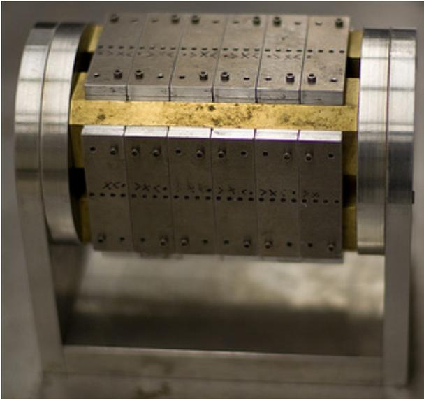
Figure 5: Manufactured undulator with all dipoles inserted.
