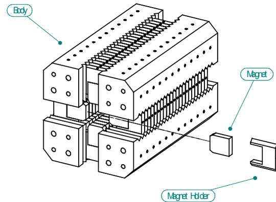
Figure 1: Undulator body and magnetic dipoles glued into their holders can slide back and forth to adjust the magnetic field  $B$ .
