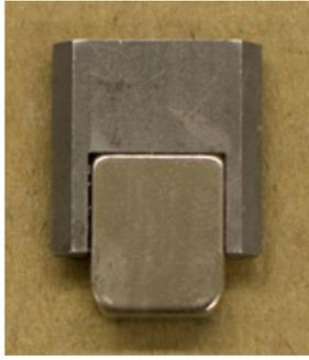
Figure 2: A completed dipole glued into its holder. Altogether there are 6 periods so 84 magnets in the undulator; 21 magnets magnetized in same direction, with 4 directions of magnetization as shown in Figure 1.
