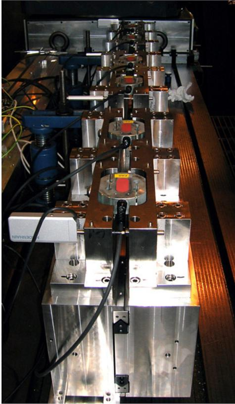
Figure 3: Stainless steel beams, phase shifting mechanism and the mechanical system used to simulate the transverse magnetic load.
