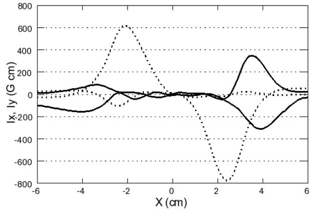
Figure 8: Field integrals at minimum gap before (dashed) and after (solid line) application of trim magnets.
