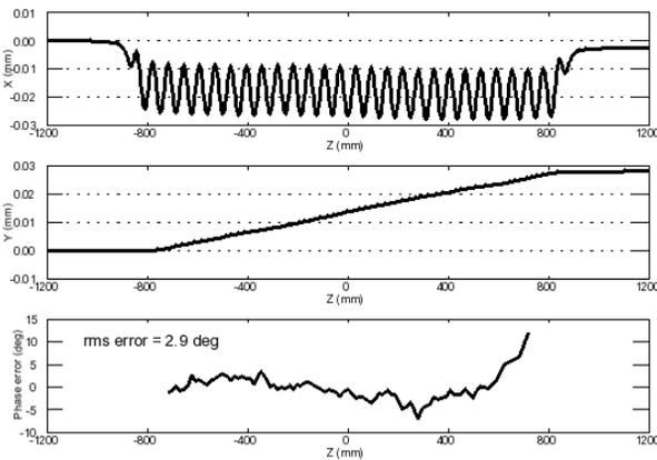
Figure 6: Trajectory and phase error at the minimum gap of 15.5 mm in horizontal polarization mode before shimming.
