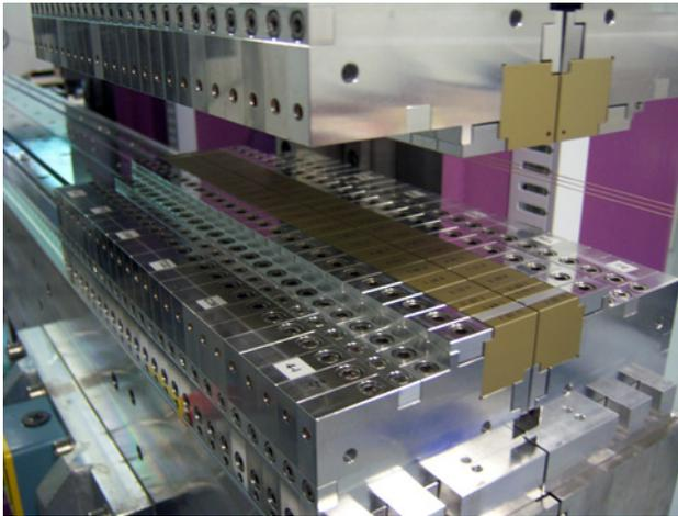
Figure 5: Partially assembled magnetic structure during the measurement/optimization process.
