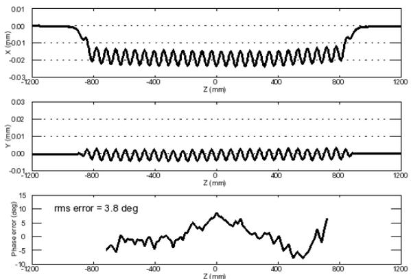
Figure 9: Trajectory and phase error in antiparallel mode at minimum gap.
