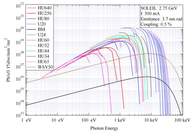
Figure 1: Average predicted brilliance of the SOLEIL insertion devices calculated using SRW [8].
