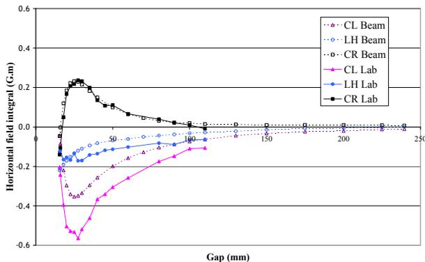
Figure 2: Comparison between the horizontal field integral from magnetic measurements and electron beam based measurements for HU52 LUCIA.
