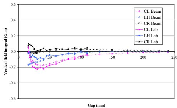
Figure 3: Comparison between the vertical field integral from magnetic measurements and electron beam based measurements for HU52 LUCIA.
