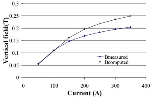
Figure 6: Comparison of measured with Bell GH701 Hall probe and computed vertical field .
