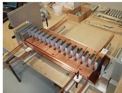
Figure 2: Assembling of the serpentine coil on the prototype.
