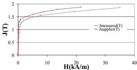
Figure 7: Magnetisation J vs magnetic field excitation H for silicon steel.
