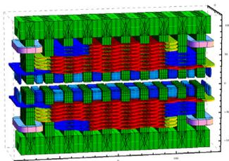
Figure 3 Radia model of a short version of the undulator (5 periods).
