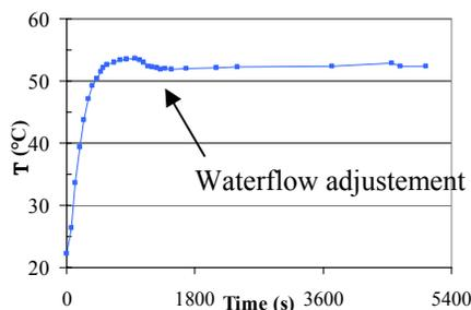
Figure 8 : Temperature with 350 A.
