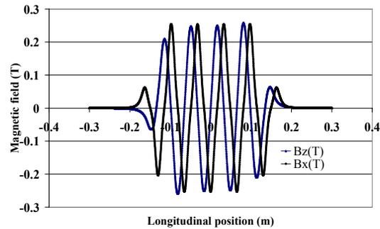
Figure 4: Computed magnetic fields at 15.5 mm gap using the RADIA model.
