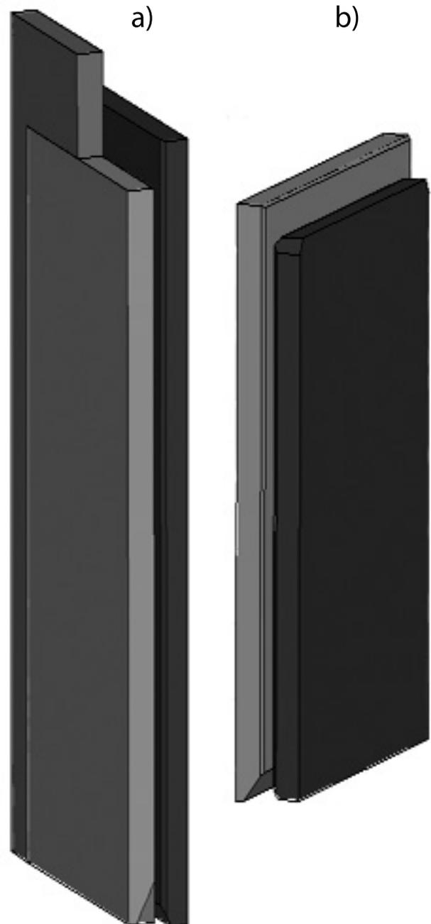
Figure 2: One quarter period of both the chimera hybrid (a) and the conventional design (b). a) Half of the SmCo sheath has been removed for viewing. The black iron pole is in the back. The chamfer of the rare earth magnet has been filled with SmCo. b) Modifications made to the magnets in Table 2 to partially mitigate large flux concentrations in the rare earth magnets.
