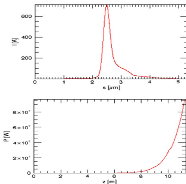
Figure 3: (Top) SPARX beam profile. The beam energy is 2 GeV. (Bottom) Laser gain of a single beam slice as a function of distance along the undulator lattice.
