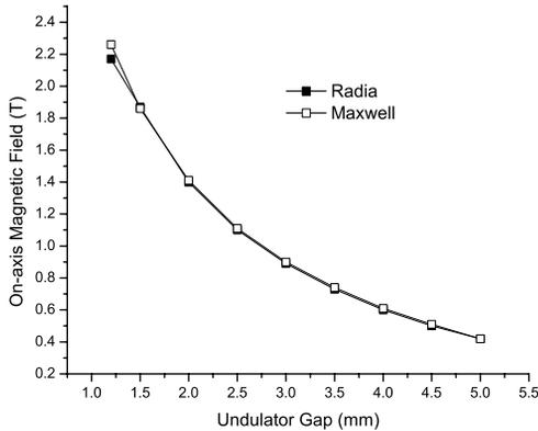
Figure 1: Calculated on-axis field for the 9mm period undulator. The divergence of the calculations at small gap is caused by the simplified geometry used in RADIA to expedite calculation.
