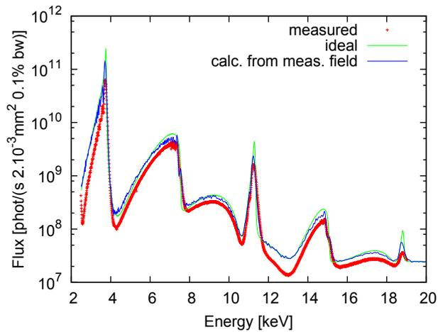
Figure 1: On-axis spectral photon flux through the  $50 \mu\text{m}$  pinhole at 14 m distance from the source for 8 mm gap and  $J_{\text{main}} = 500 \text{ A/mm}^2$ : measured, calculated from an ideal and from the measured SCU14 field map.
