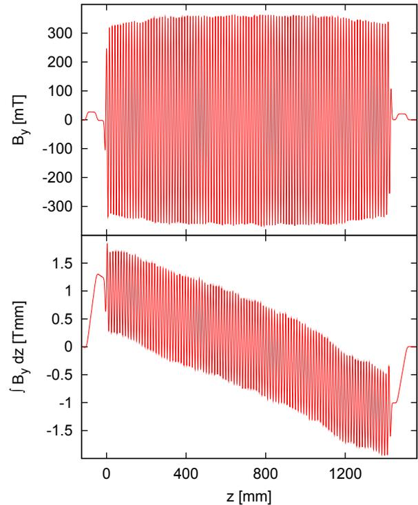
Figure 3: Measured field and first field integral map of the SCU14 for 8 mm gap and  $J_{\text{main}} = 500 \text{ A/mm}^2$ .
