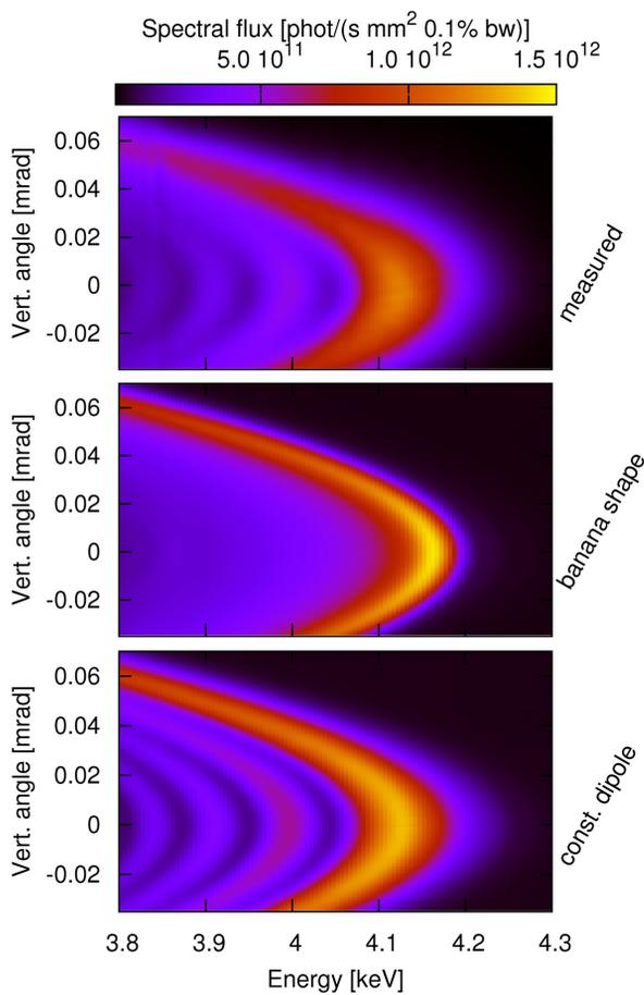
Figure 4: Vertical angular spectral distribution of the photon flux for 16 mm gap and  $J_{\text{main}} = 400 \text{ A/mm}^2$ : measured (top) and calculated from simulated field maps reflecting the systematic field amplitude decrease ("banana shape"-error, middle) and the constant dipole field error (bottom).
