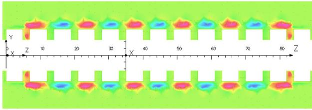
Figure 4: Close-up on eddy currents formed in iron yokes during current ramp. Red areas indicate current in positive x-direction (inwards), blue areas in negative x-direction. Note the large end pole eddy currents.
