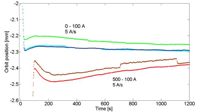
Figure 3: Drift at 100 A after up-ramp (0-100 A, upper curves) and down-ramp (500-100A, lower curves).
