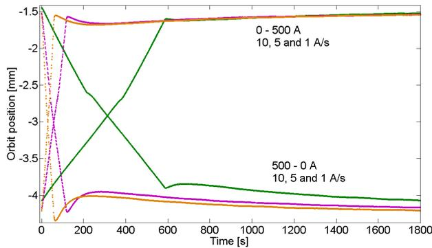
Figure 2: Ramp rate dependence for positive and negative ramps.
