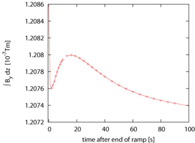
Figure 5: Time variation of the 1st field integral after an up-ramp, caused by eddy currents in the iron yokes.
