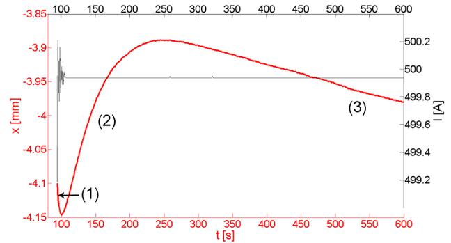
Figure 1: Drift curve during and after a 100-500 A ramp. Transient parts seen are 1. a small overshoot followed by 2. a large and steep decay, and lastly 3. a slow increase towards stabilization. The upper curve shows the corresponding current.
