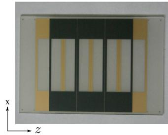
Figure 4: Photograph of the set of seven correction loops. Two  $500\ \mu\text{m}$  thick sapphire substrates are sputtered with four and three YBCO loops with a thickness of  $330\ \text{nm}$ , covered with a  $200\ \text{nm}$  thick gold layer. Dimensions of the loops:  $14\ \text{mm} \times 44\ \text{mm}$ . The two substrates are stacked and mounted at a distance of  $1\ \text{mm}$  from the surface of the undulator.
