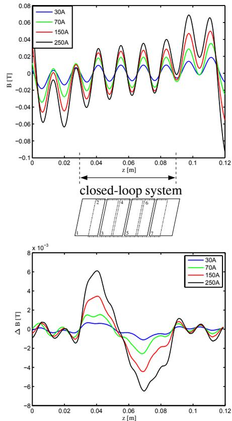
Figure 5: The influence of the YBCO closed loop system on the field shown in Fig. 2 for various undulator currents (above) and the difference of the field measurements with and without the YBCO loops system (below). The YBCO loop system tries to compensate the field which increases from left to right in Fig. 2.
