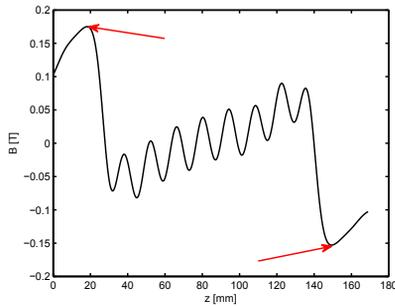
Figure 2: The distorted magnetic field strength of an undulator mock-up before applying the induction shimming concept. The field is significantly deformed by the end plates (red arrows).
