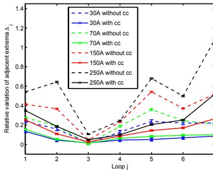
Figure 6: Ratio of the absolute values of adjacent extrema with and without the YBCO loop system for different currents  $I_{main}$ . The values at the beginning and the end are higher due to the finite length of the induction-shimming system.
