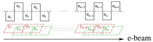
Figure 1: Concept of induction-shimming. The sinusoidal field in one of the undulator-halves is approximated for the sake of simplicity by a rectangular shape. Due to minor field errors caused by finite tolerances the amplitude of the field varies slightly. This variation is compensated by HTSC loops (red and green). The length of one loop in the beam direction is exactly one ideal period length.
