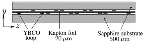
Figure 3: Cut through the stacked induction-shimming structure with the substrate. The YBCO loops are arranged on a  $500\ \mu\text{m}$  thick sapphire substrate. The thickness of the YBCO layer is  $330\ \text{nm}$ . The period of the mock-up is  $14\ \text{mm}$ .
