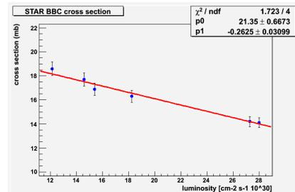
Figure 5: STAR BBC effective cross section as a function of pp luminosity .
