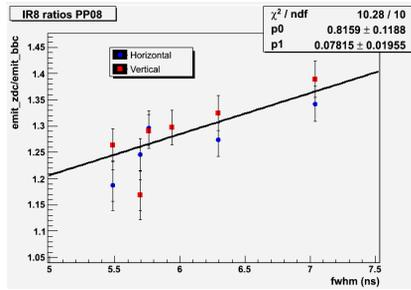
Figure 2: Ratio of emittance measured by the ZDC and the emittance measured by the BBC in PHENIX as a function of the FWHM of the overlap region of both beams. The BBC emittance is derived after a  $\pm 30$  cm vertex cut.
