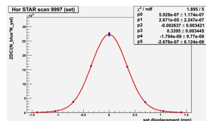
Figure 1: Vernier scan in STAR using the ZDCs in the horizontal plane.
