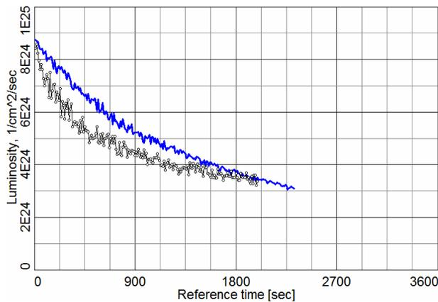
Figure 1: Simulation of full luminosity for 56 bunches  $\gamma=6.3$  ( $\beta^*=10\text{m}$ ,  $\epsilon=15 \mu\text{m}$ ,  $N=1 \times 10^9$ ,  $S_{95\%}=0.2\text{eV-s/n}$ ): 1) blue upper curve – 56 MHz RF (2.5 MV); 2) black lower curve – 28 MHz RF (0.5 MV).
