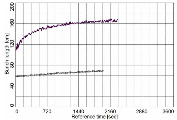
Figure 2: RMS bunch length at  $\gamma=6.3$  ( $\epsilon=15 \mu\text{m}$ ,  $S_{95\%}=0.2\text{eV-s/n}$ ,  $N=1 \times 10^9$ ): 1) upper curve – 28 MHz RF (0.5 MV gap voltage); 2) lower curve – 56 MHz RF (2.5 MV).
