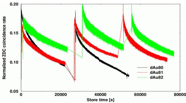
Figure 4. Comparison of normalized ZDC collision rates for the original configuration (dAu80,  $\beta^*=1\text{m}$  in blue and yellow), for the yellow squeeze (dAu81,  $\beta^*=1\text{m}$  in blue and  $\beta^*=0.7\text{m}$  in yellow) and for both rings (dAu82) at  $\beta^*=0.70\text{m}$ .
