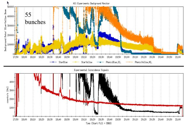
Figure 6. Collimation and collision steering during the test of 0.65m optics in P-P with a 56 bunches physics store.
