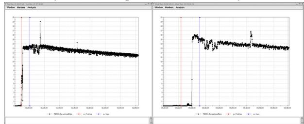
Figure 3. Comparison of normalized (for total intensity) collision rates for 1m  $\beta^*$  (left) and 0.70m (right) in the expected 15% ratio.
