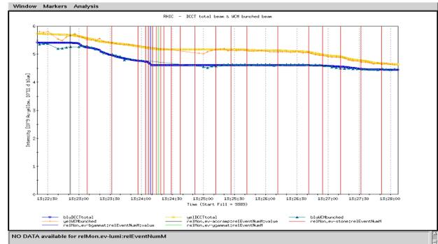
Figure 1. First successful ramp with  $\beta^* = 0.7\text{m}$  in yellow.
