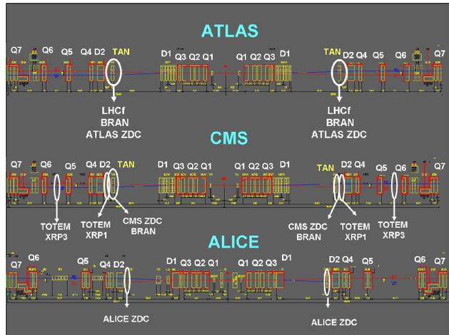
Figure 2: The forward detectors inside the Long Straight Sections.
