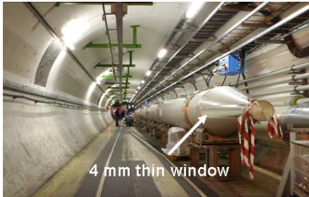
Figure 6: Big circular chamber in front of ALICE ZDC.
