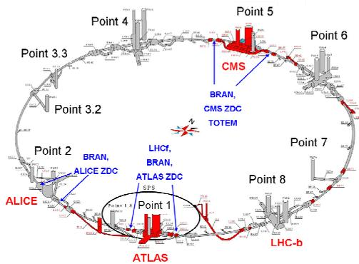
Figure 1: The forward detectors around the LHC.
