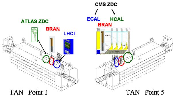
Figure 3: The forward detectors inside the TANs
