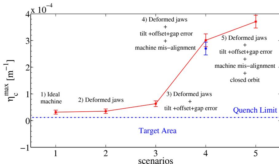
Figure 1:  $\eta_c^{max}$  for multiple combinations of collimator and machine imperfections at collision energy. The blue point refers to machine alignment errors as defined by measurements. The cleaning efficiency gets worse up to a factor of 11 by reducing  $I_{max}$  to  $<5\%$  of  $I_{nom}$ .
