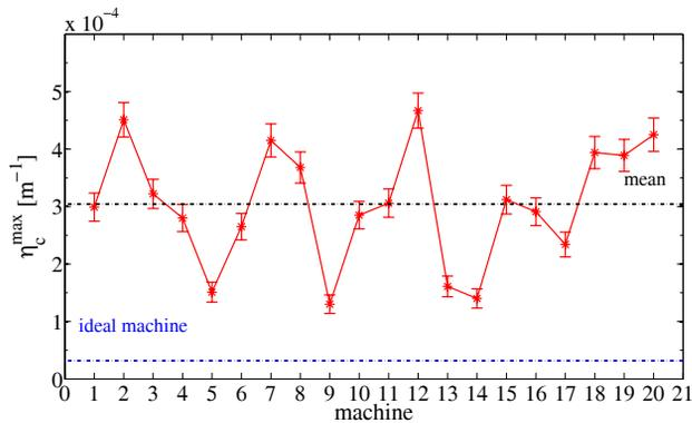
Figure 2: Cleaning inefficiency  $\eta_c^{max}$  for 20 different seeds of machine alignment errors (design values).  $\eta_c^{max}$  is increased on average by a factor of 9.5 with respect to the ideal machine.
