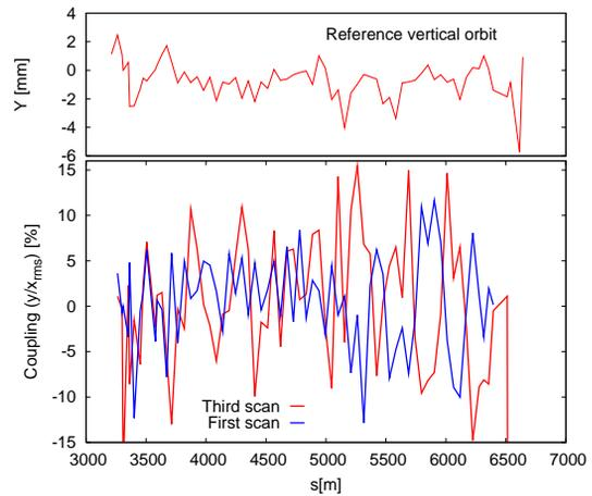
Figure 7: Vertical reference orbit (top) and coupling coefficient (bottom) versus longitudinal position during two horizontal oscillations
