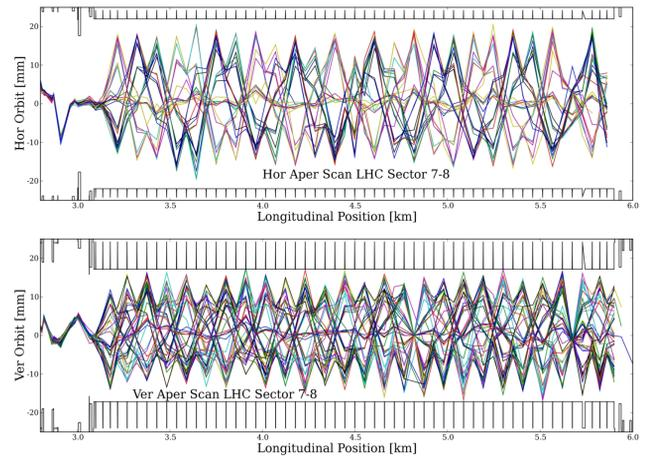
Figure 4: Measured trajectories of the injected beam 2 during the aperture scans in the LHC sector 7-8. Longitudinal (counter-clockwise) position from point 1 is given.
