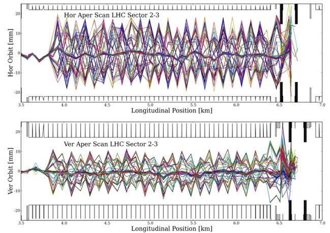
Figure 3: Measured trajectories of the injected beam 1 during the aperture scans in the LHC sector 2-3. Longitudinal (clockwise) position from point 1 is given.
