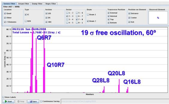
Figure 5: Beam losses recorded in arc 7-8 for a horizontal oscillation amplitude of 19 nominal beam  $\sigma$ .
