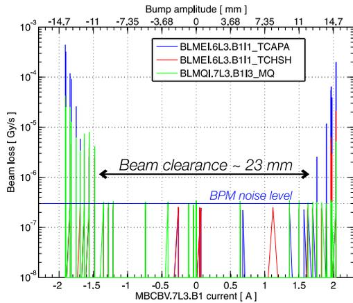
Figure 6: Beam losses versus bump amplitude (top axis) during the local aperture scan at MQ.7L3.B1. The MBCBV.7L3 corrector current is given in the bottom axis.
