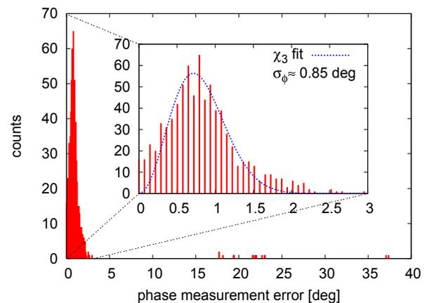
Figure 2: Phase measurement error in the SPS.
