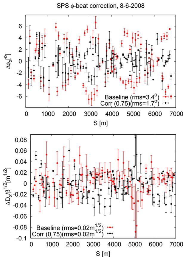
Figure 6: Phase (middle) and normalized dispersion (bottom) beatings before and after correction for the measurements on the 8<sup>th</sup> of June, 2008. The top 2 plots show the variation of the horizontal orbit and the orbit corrector strengths used for the correction.
