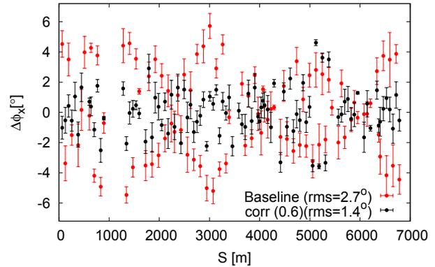
Figure 7: Phase beatings before and after correction for the measurements on the 6<sup>th</sup> of June, 2008, showing the repeatability of the correction.
