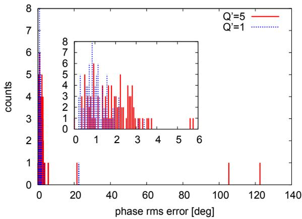
Figure 3: Phase measurement error in the SPS for the chromaticities of 1 and 5.
